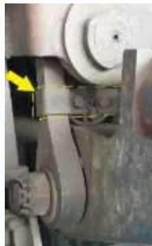
Image - safety collar applied on pendulum arm (model)
